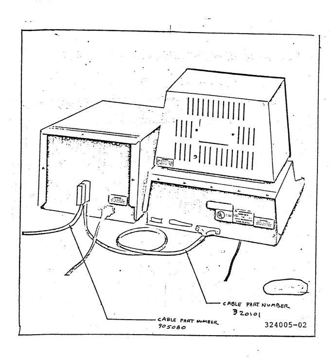
Figure 2-1. System Interconnection Diagram.
